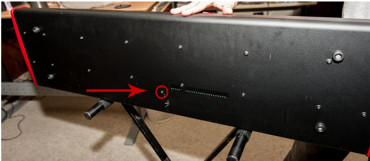
Figure 1 – First screw removal
