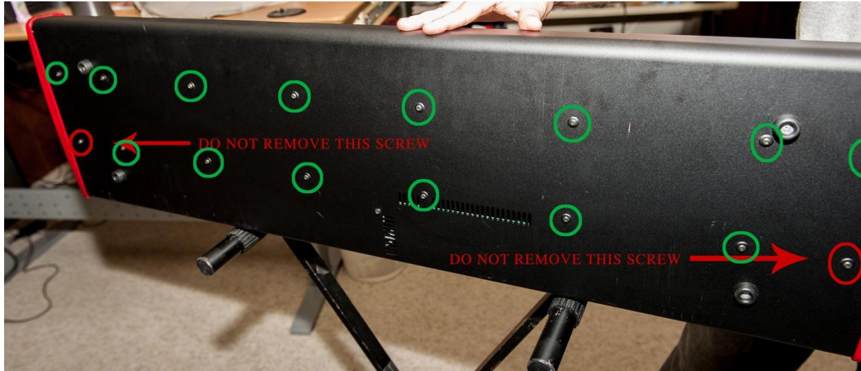
Figure 6 - Key bed screw removal
